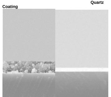
Fig. 4 Nano particle layer. Fig. 5 meso-porous layer
