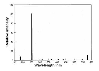
Fig.1. Spectrum of mercury low pressure discharge (100% level is 254 nm line)
