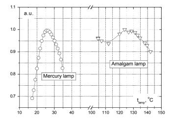
Fig.2. Relative UV output depending on liquid mercury or amalgam temperature.
