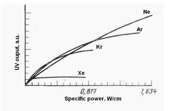
Fig.3 UV output depending specific power for different ballast gases.
