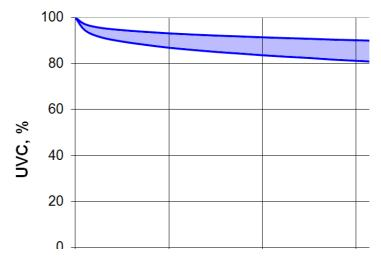
Fig6. Typical curves of UV output drop for powerful amalgam lamps.
